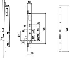
SINGLE POINT LOCK. In compliance with UNI EN 14846 standard. Flat STAINLESS steel front plate section mm 25x3, length mm 536. **Supplied with:** Control unit. Connecting cables. Fixing screws. Splitted handle follower.
