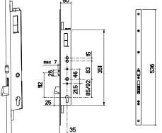
SINGLE POINT LOCK. In compliance with UNI EN 14846 standard. Flat STAINLESS steel front plate section mm 25x3, length mm 536. Supplied with: Control unit. Connecting cables. Fixing screws. Handle follower.
