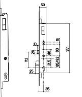
SINGLE POINT LOCK. In compliance with UNI EN 14846 standard. Flat STAINLESS steel front plate section mm 25x3, length mm 536 **Supplied with:** Control unit. Connecting cables. Fixing screws.
