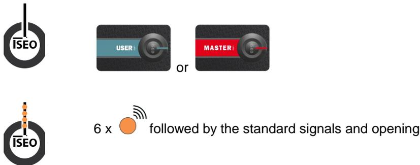
The mechanical override usage signal stays until it will be reset.
