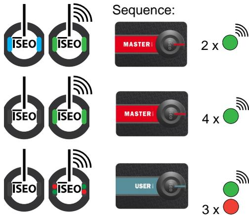
**Deleting all the channels and clearing the White List (PAD ACD)**
