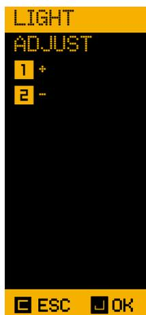
The keyboard's light can be adjusted from off to maximum luminosity, in 8 different degrees, by pushing button 1 to increase and button 2 to decrease luminosity. A sequence of three short acoustic signals close to each other, indicates that maximum or minimum luminosity has been reached.
