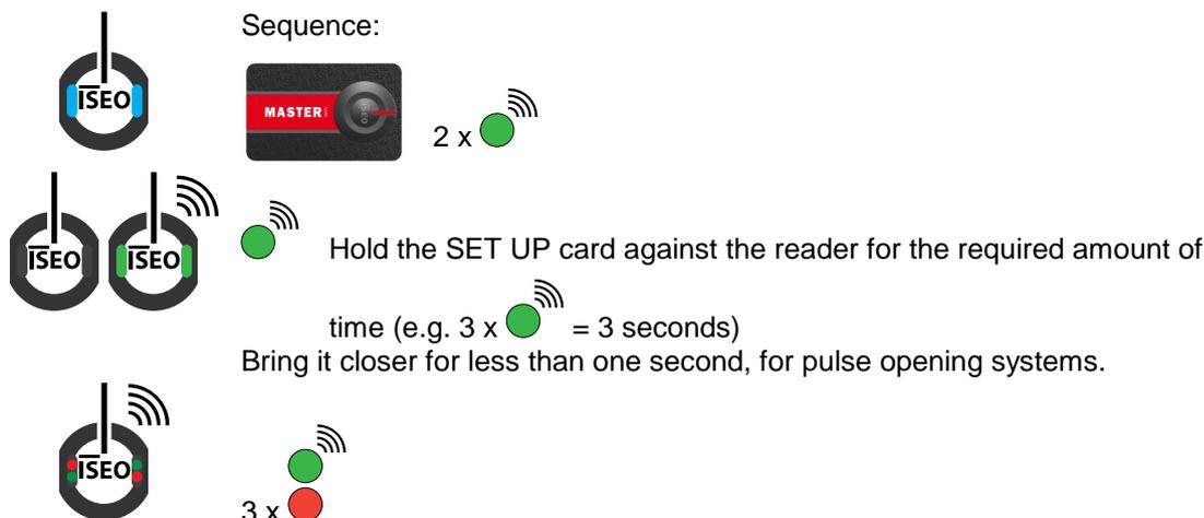
Hold the SET UP card against the reader for the required amount of time (e.g. 3 x
